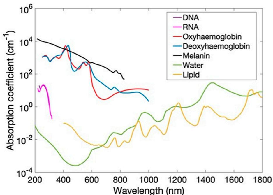
**Figure 1.** Absorption coefficient spectra ( $\mu a$ ) of endogenous tissue chromophores, including DNA, RNA, oxyhemoglobin, deoxyhemoglobin ( $150 \text{ g L}^{-1}$ ), melanin, water, and lipid. Adapted with permission from T. Zhao, A. E. Desjardins, S. Ourselin, T. Vercauteren, W. Xia, *Photoacoustics*, Vol.16, Article ID100146, 2019; licensed under a Creative Commons Attribution (CC BY) license.
