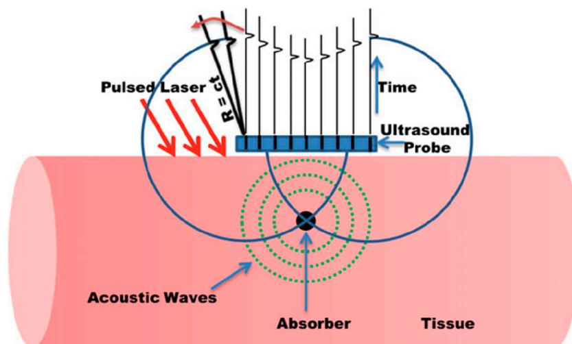
**Figure 3.** Back-projection PAI reconstruction for a planar detection geometry. Reproduced with permission from Handheld Probe-Based Dual Mode Ultrasound/Photoacoustics for Biomedical Imaging. In: Olivo M., Dinis U. (Eds) *Frontiers in Biophotonics for Translational Medicine*. Progress in Optical Science and Photonics, volume 3. Springer, Singapore (2016). Copyright 2016 Springer, Singapore.
