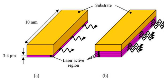
**Figure 13.** Schematic diagram of (a) a standard diode bar and (b) a multiple active region diode bar. Adapted with permission from Proc. SPIE 9887, Biophotonics: Photonic Solutions for Better Health Care V, 98872B (2016). Copyright 2016 Society of Photo-Optical Instrumentation Engineers (SPIE).
