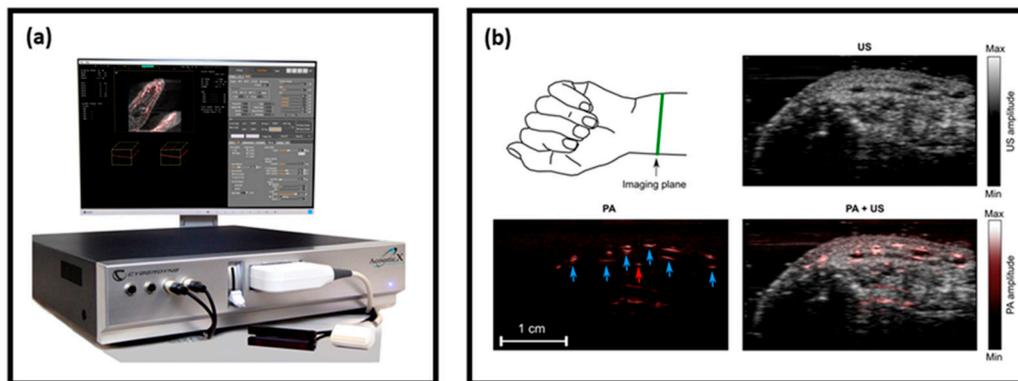
**Figure 9.** (a) Photograph of the LED-based PA and US imaging system—AcousticX; (b) US (gray colormap), PA (hot colormap), and US/PA overlay cross-section images of a human volunteer’s wrist acquired at a frame rate of 10 Hz. Blood vessels are marked using blue arrows in the PA image. Adapted with permission from W. Xia, M. Kuniyil Ajith Singh, E. Maneas, N. Sato, and A. E. Desjardins, *Sensors*, Vol.18, Article ID1394, licensed under a Creative Commons Attribution (CC BY) license.
