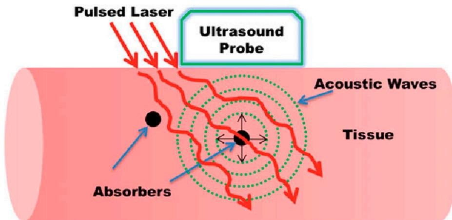
**Figure 2.** Basic principle of biomedical photoacoustic imaging. Reproduced with permission from Handheld Probe-Based Dual Mode Ultrasound/Photoacoustics for Biomedical Imaging. In: Olivo M., Dinisch U. (eds) *Frontiers in Biophotonics for Translational Medicine. Progress in Optical Science and Photonics*, vol 3. Springer, Singapore (2016). Copyright 2016 Springer, Singapore.
